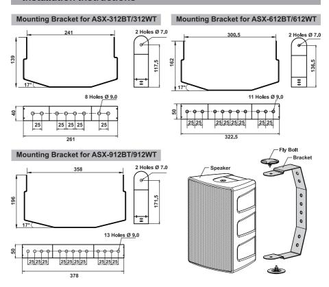
The speaker system is supplied with specially designed mounting bracket. It helps in the installation of this speaker system in three positions i.e, Vertical, Horizontal and Inclined.
